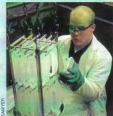
A technician inspects cultured x-plate quartz crystals. The orientation of the birefringent axes in these crystals make them well suited for use as large optical waveplates.
