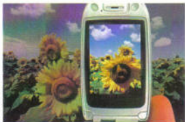
FIGURE 1. Electronic displays generally must compromise natural brightness to retain deep color saturation (background). A display system designed around human visual processes, however, can retain brightness as well as color saturation (foreground).
