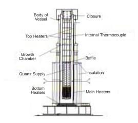
After sealing the vessel, the autoclave is heated to operating conditions with the use of external, resistance heaters. Typical operating conditions are between 300 and 400°C. The internal pressure developed is controlled by the temperature and the amount of solution added to the autoclave.
